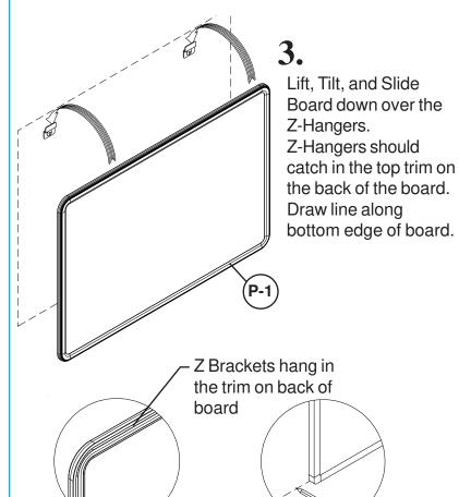
Lift and remove board from the Z-Hangers. Measure up from bottom line of board 1-1/8", and draw line as shown. Locate stud near each end of board and drill pilot hole along line using 1/8" drill bit.
