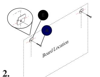
Attach Z-Hangers (E) using Long Screws (A) as shown.
