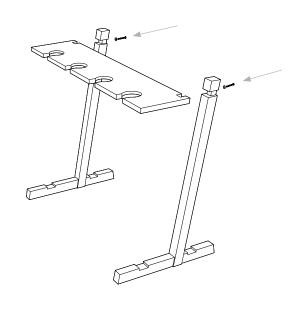
2. Insert each rail into place with cork facing inward and secure using x4 long bolts with washers.
