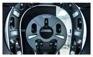
"The cameras have to be in a specific spot at a certain angle," says Boyer. KYDEX® Thermoplastics pieces have to line up perfectly with the cameras, so some have unusual undercuts, and the bends and cutouts are intricate."
