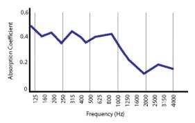
Absorption Coefficients and Noise Reduction Coefficient for the product were measured by an independent, accredited NVLAP facility according to the test methods as defined by ASTM C 423 and ASTM E 795. Random incidence Absorption Coefficients for the product in an E-400 mounting shall be as follows:
