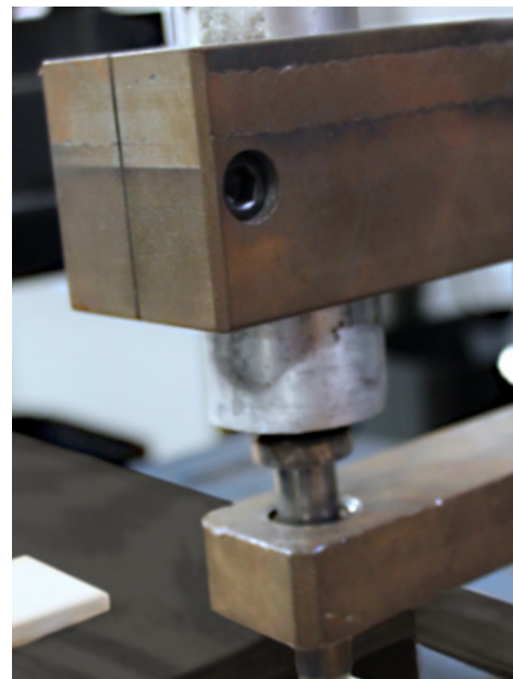
At top: Falling weight drop dart test with GE geometry: the smallest outer diameter and largest rounded metal head.
